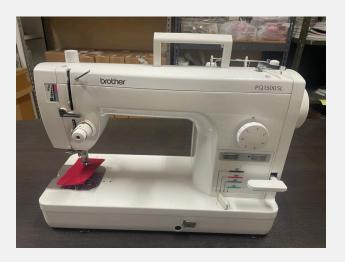
The Brother PQ1500SL is a high-speed straight stitch machine, perfect for serious quilters and dedicated seamstresses. It sews up to 1,500 stitches per minute with four feed dog settings to give you total control over all types of fabric, from delicate silks to heavy quilts. The adjustable pin feed system gives you smooth, even fabric feeding without leaving marks and a built-in knee lifter lets you raise the presser foot hands-free for seamless repositioning.
